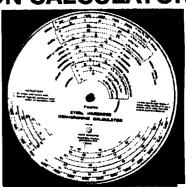
All the recognized hardness scales are incorporated, including: Brinell (steel or Tungsten-carbide ball), Firth, or Vickers, Monotron, Herbert Pendulum, Scelerescope, Knoop, Rockwell 'B', Rockwell 'C', Rockwell Superficial 30N, and Rockwell Superficial 30T.
