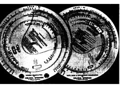
sizes to be determined very rapidly as the Rate and Stress for a particular spring can be read off in a few seconds by setting the dials to the appropriate values.
